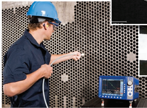
Conco NDE Technician Using MIZ28 Multi-Frequency Analyzer.
